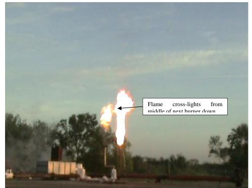
Figure 3 - Multi-point flare cross lighting relies on hot-combustion gases (radicals) from the piloted burner to ignite the neighboring burner
