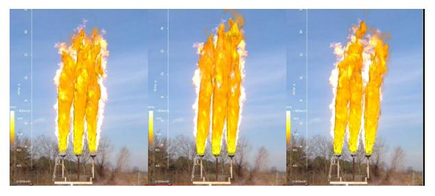
Figure 4 - Comparison of predicted and measured flame shape for a 3-Flare Test burning ethylene gas [15]
