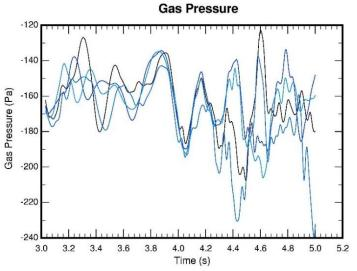
Figure 16 - Pressure wave created with ignition under a 20mph wind blowing parallel to the lit row
