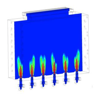
During normal operation, Low-emission burner flames are more affected by furnace currents which can extinguish the flame allowing fuel gas to collect in one region of the furnace box. With oxygen from another part of the furnace transported to the fuel rich region, a large flame may result creating a over-pressure condition in the furnace box that disrupts steady operation, leads to non-optimal performance and can even damage process tubes in the convection section above the furnace box.
