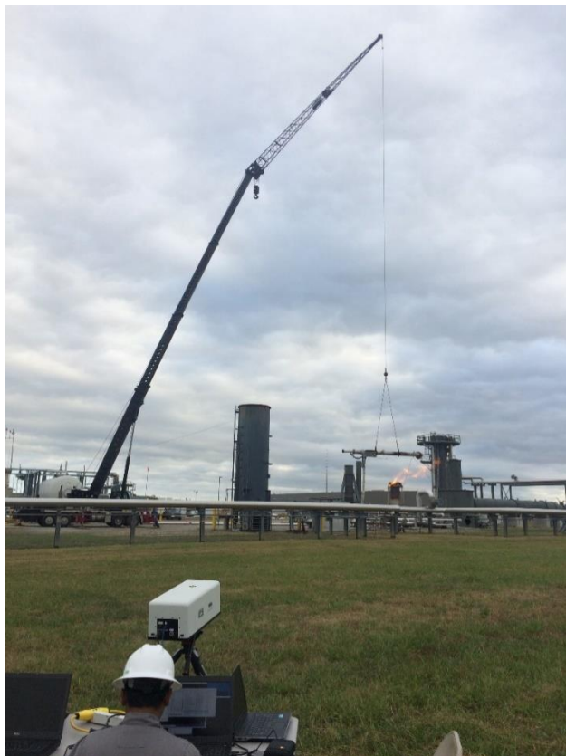
Figure 2: Typical VISR setup during the Test.
